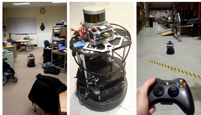
(a) The office area used for collecting training data. (b) The modified Turtlebot robot used for data collection. (c) The open lab area used for collecting training data.
